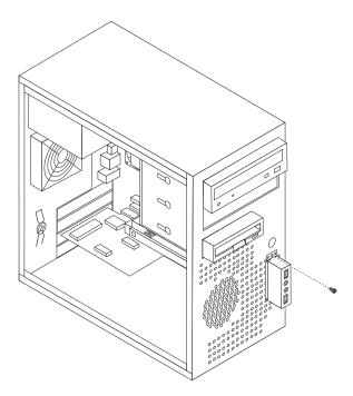
Figure 32. Removing the front audio and USB assembly
